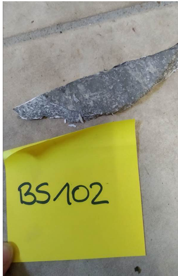
Asbestzementplatte Heizraum [BS102]
